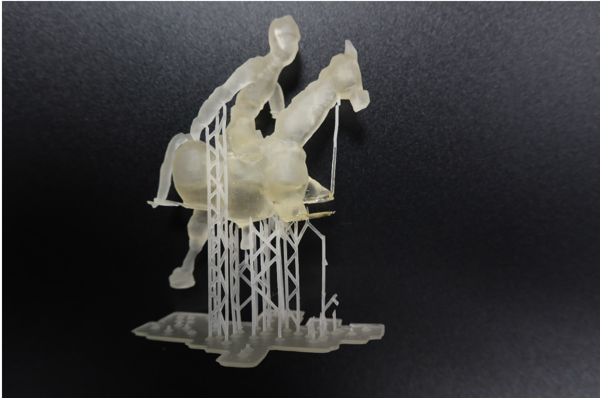
Figure 10 Insufficient support structure
