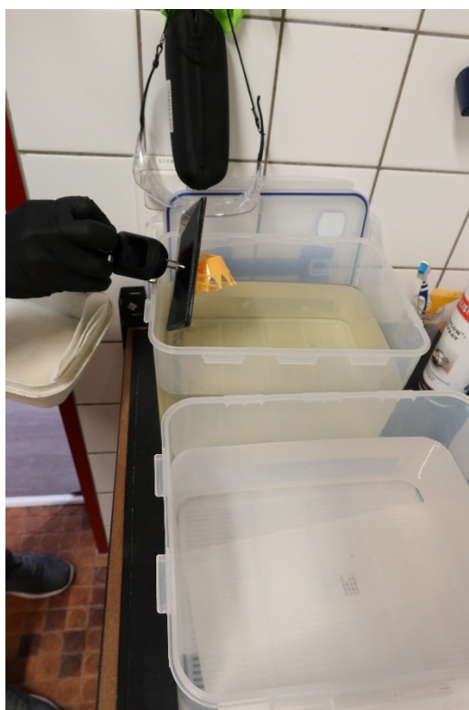
Figure 4 Placing the building plate in the cleaning bath
