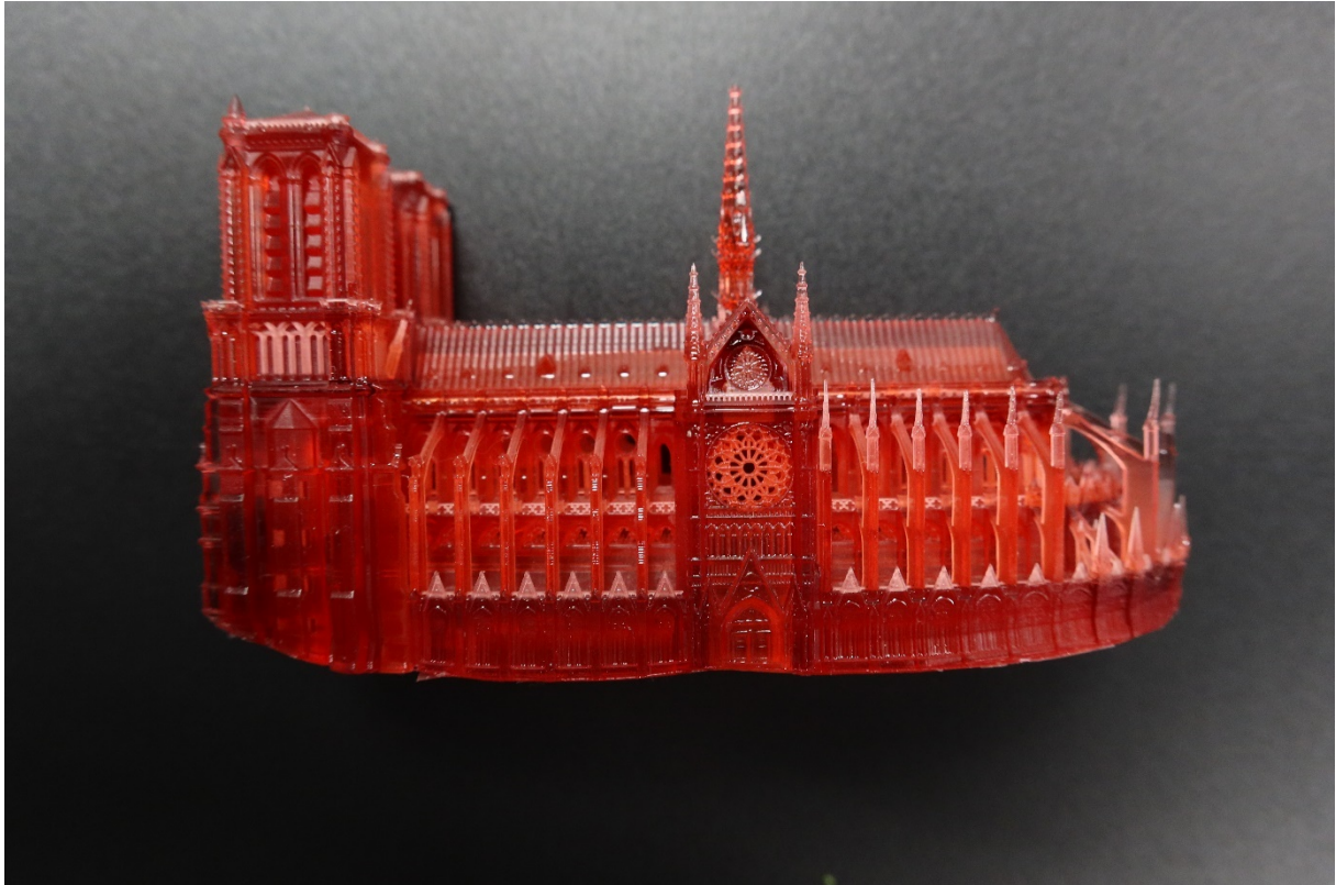
Figure 11 Deformation due to incorrect positioning and insufficient support material at the edges
