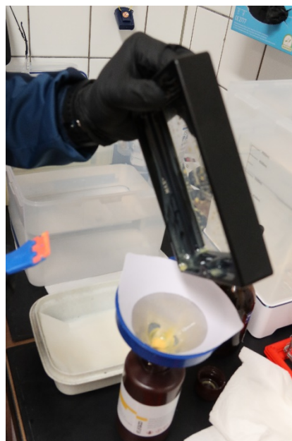
Figure 6 Refilling the resin
