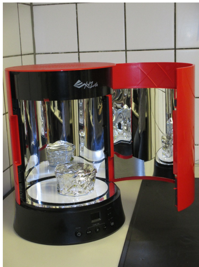
Figure 9 Curing chamber (example XYZ Printing) with mirror unit
